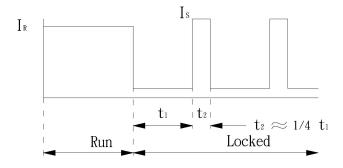
3rd wire signal Run : Square Wave Locked : V∏or V∟
