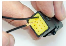
2. Insert the crimped contacts through the single wire seal into the contact chambers.
