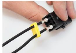
2. Crimp the contacts and insert them into the contact chambers.
