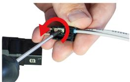
2. Loosen the screws on the contact carrier.
