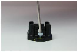
1. Fasten the bulkhead mounted housing with two M3 screws, tightening torque: 0.25 Nm.
