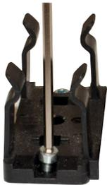
1. Fasten the mounting frame on the installation surface. Tightening torque is 0.3 Nm.
