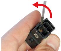
1. Lever the contact carrier out of the Han® 1A insulation body.
