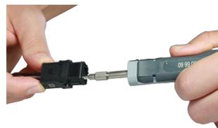
2. Remove Han D® contacts by using the removal tool 09 99 000 0012.
