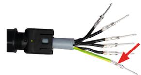
2. Check the crimp quality through the inspection holes of the terminals!
