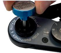
5. Secure the position sleeve with the safety clip (optional).
