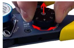
8. To replace the position sleeve, remove the safety clip and follow point 4 in reverse order.
