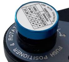
7. With the tool fully open, raise the selector knob and turn it to the appropriate position (arrow points to the selected setting).
