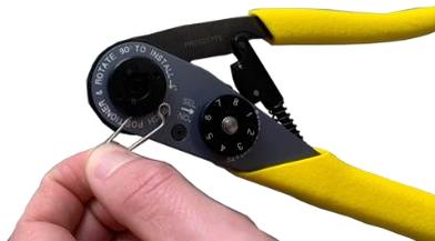
3. Select the position sleeve required for the contact.
