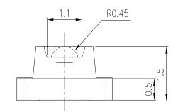
For reflow soldering (propose)
