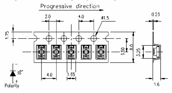
**Note:** The tolerances unless mentioned are  $\pm 0.1$ , Unit = mm.
