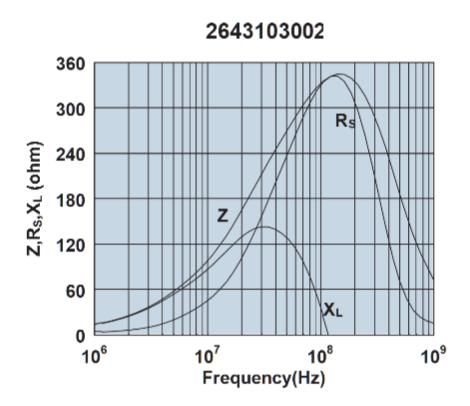
Impedance, reactance, and resistance vs. frequency.
