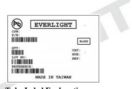
Tube Label Explanation CPN: Customer's Product Number P/N: Product Number QTY: Packing Quantity CAT: Rank of (VF)(Note\*1)(Note\*2) Note1:  $\lambda_d$ /CIE/Color temperature Note2: Luminous Intensity/ Total Flux HUE/REF: Reference LOT No: Lot Number
