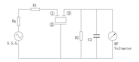
$\begin{array}{ccc} R1{=}280\,\Omega\,{\pm}5\%, R2{=}330\Omega{\pm}5\%, Rg{=}50\Omega & \text{(1):Input} \\ C2{=}10\,Pf \text{(Including stray capacitance} & \text{(2):Ground} \\ \text{and capacitance of RF Voltmeter)} & \text{(3):Output} \\ S.S.G:Output \,Voltmeter & \text{(3)} \end{array}$
