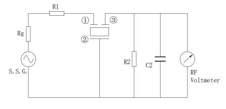
$\begin{array}{l} R1+Rg = R2 = 330\Omega \pm 5\%, Rg = 50\Omega \\ C2 = 10 \ PF \ (Including \ stray \ capacitance \ and \ capacitance \ of \ RF \ Voltmeter) \\ S.S.G: Output \ Voltmeter \end{array}$
