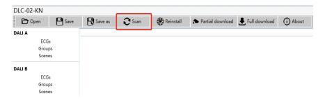
Note: During the first time installation, "Scan" and "Reinstall" make a no difference in searching devices and addressing. After an installation, the "Scan" button carries out a search for previously addressed and unaddressed devices. Addressing for previously addressed devices will remain unchanged. The next available address is then assigned to devices which have been recently added, whereas "Reinstall" removes all addresses and then re-addresses them.
