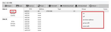
Command 1: ECG-on Turn on the ECG.
