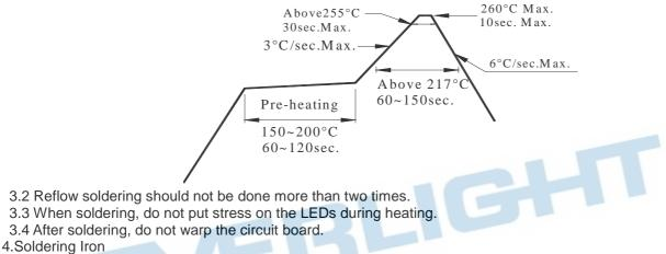
Each terminal is to go to the tip of soldering iron temperature less than 350°C for 3 seconds within once in less than the soldering iron capacity 25W. Leave two seconds and more intervals, and do soldering of each terminal. Be carefu because the damage of the product is often started at the time of the hand solder.
