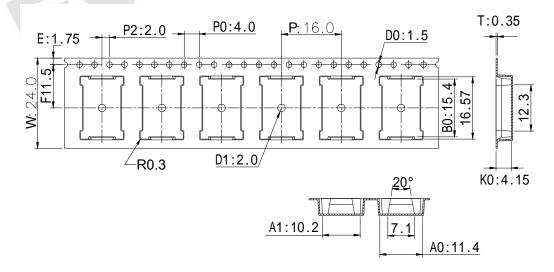
Note: Tolerances unless mentioned  $\pm 0.25$ mm. Unit = mm
