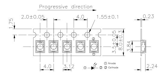
TOLERANCES UNLESS DIMENSION±0.1 ANGLE±0.5 UNIT:mm
