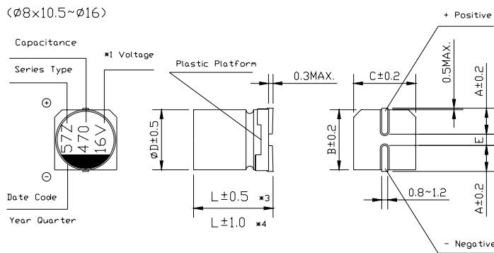
\*1 Voltage mark [6V] represents 6.3V for  $\Phi 4 \sim \Phi 10$ ;
