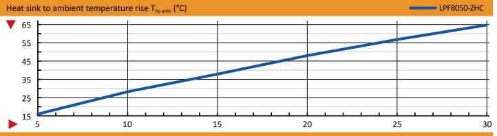
Dissipated Power Pd(W)
