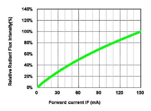
Fig.4. Forward Current vs. Relative Radiant Flux
