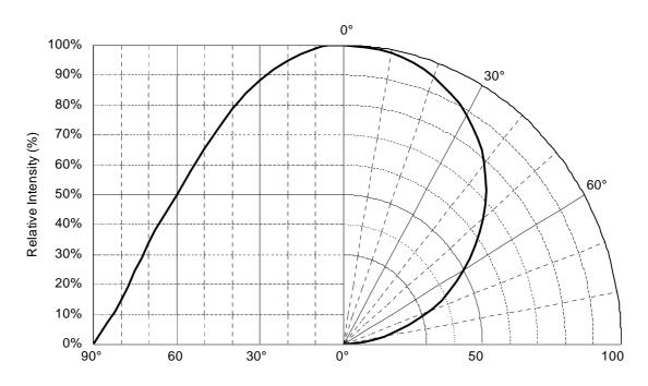
Fig2. Radiation Characteristics
