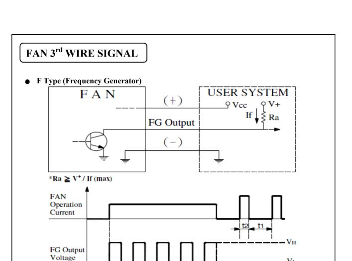
★Electrical Characteristics : (at Ta = 25°C, Vcc = Rated Volt.)
