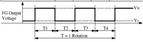
T=T1+T2+T3+T4=1 Rotation  $T=\frac{60}{\text{rpm}}$
