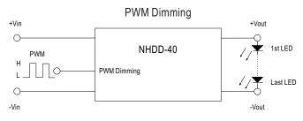
H: >1.5~5VDC or open circuit L: <0.9VDC or short
