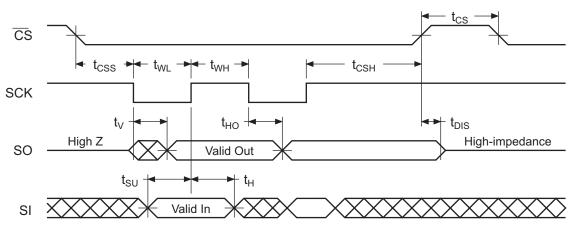
Figure 31. Waveform 2 = SPI Mode 3 Compatible
