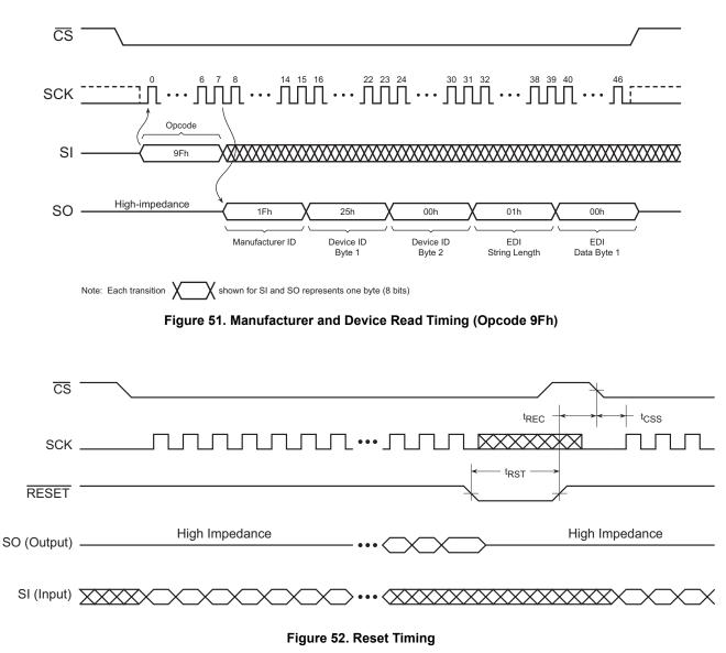
Note: The CS signal must be in the high state before the RESET signal is deasserted.
