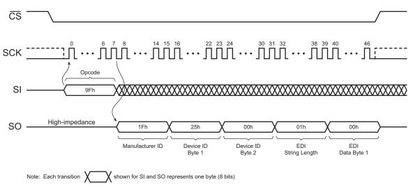
Figure 22. Read Manufacturer and Device ID
