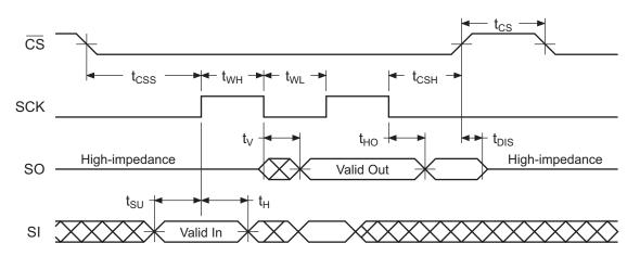
Figure 30. Waveform 1 = SPI Mode 0 Compatible
