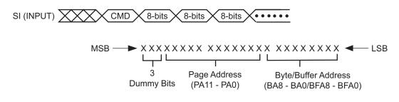
Figure 29. Command Sequence for Read/Write Operations for Page Size 264 bytes (Except Status Register Read, Manufacturer and Device ID Read)
