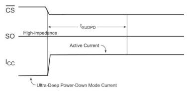
Figure 20. Exit Ultra-Deep Power-Down (Chip Select Low)
