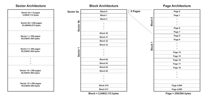
Figure 3. Memory Architecture Diagram
