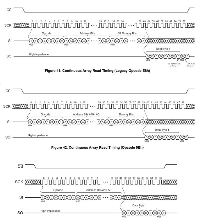
Figure 43. Continuous Array Read Timing (Opcode 01h or 03h)
