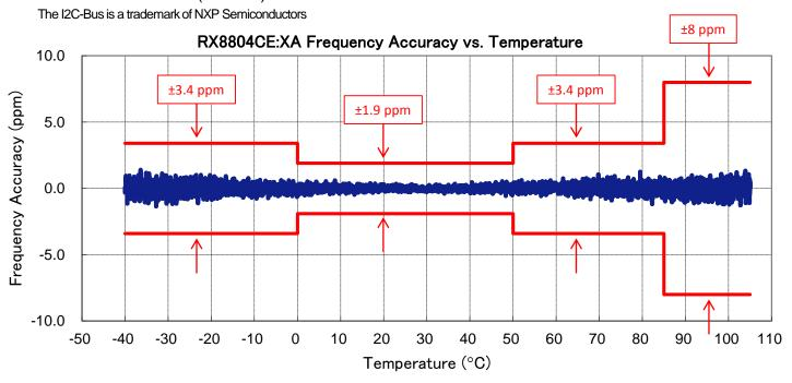
Designed for precision time keeping, Epson's RX8804CE uses Digitally Temperature-Compensated Crystal Oscillator (DTCXO) technology to achieve  $\pm 3.4$  or  $\pm 8$  ppm accuracy over temperature of -40 to +85 °C or -40 to +105 °C respectively, equivalent to  $\pm 9$  or  $\pm 20$  seconds per month. Compared to RTCs integrated into microcontrollers (MCUs), Epson's RX8804CE includes an integrated crystal, is lower power, and is far more accurate.
