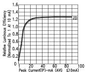
0 1 20 40 60 80 100 Peak Current(IP)-mA (AVG ≤10mA) Fig2. RELATIVE LUMINOUS EFFICIENCY LUMINOUS INTENSITY PER UNIT CURRENT) VS. PEAK CURRENT
