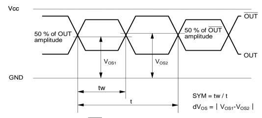
Differential output waveform (OUT - OUT)
