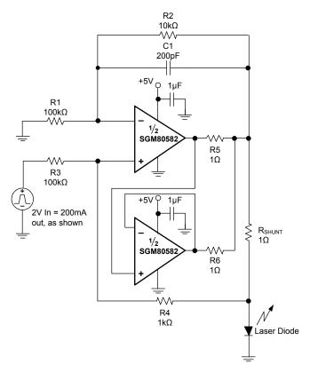
Figure 3. Parallel Operation
