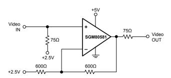
Figure 4. Single-Supply Video Line Driver
