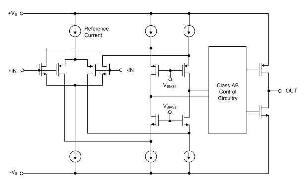
Figure 1. Simplified Schematic
