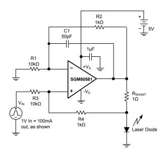
Figure 2. Laser Diode Driver
