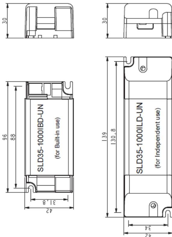
• With terminal cover and cable clamp, the power supply can be independent installed.
