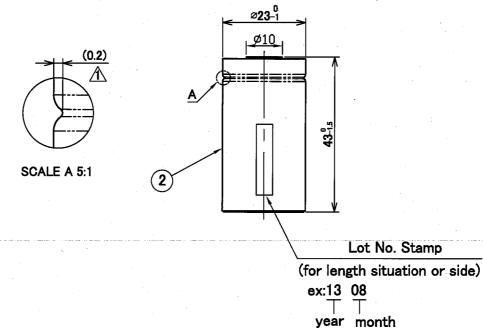
**NOMINAL VOLTAGE: 1.2 V** RATED CAPACITY : 2800 mAh AVERAGE CAPACITY: 3050 mAh
