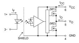
Note: A 0.1- $\mu F$  bypass capacitor must be connected between pin 6 and pin 4.
