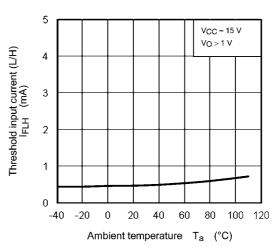
Fig. 13.2.4 I<sub>FLH</sub> - T<sub>a</sub>
