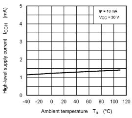
Fig. 13.2.6 I<sub>CCH</sub> - T<sub>a</sub>
