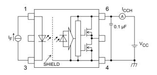
Fig. 13.1.5 I<sub>CCH</sub> Test Circuit
