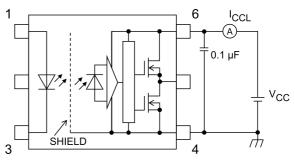
Fig. 13.1.6 I<sub>CCL</sub> Test Circuit
