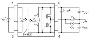
Fig. 13.1.4 V<sub>OL</sub> Test Circuit
