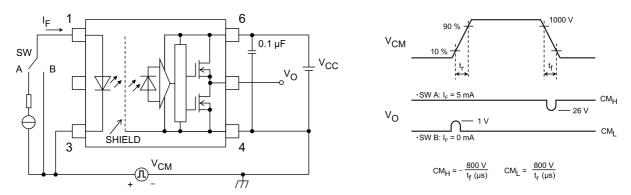
Fig. 13.1.8 Common-Mode Transient Immunity Test Circuit and Waveform
