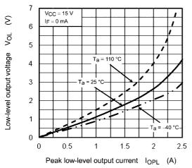
Fig. 13.2.9 V<sub>OL</sub> - I<sub>OPL</sub>
