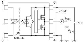
Fig. 13.1.1 I<sub>OPH</sub> Test Circuit
