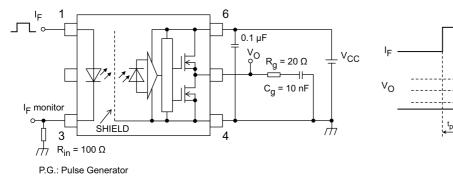
Fig. 13.1.7 Switching Time Test Circuit and Waveform
