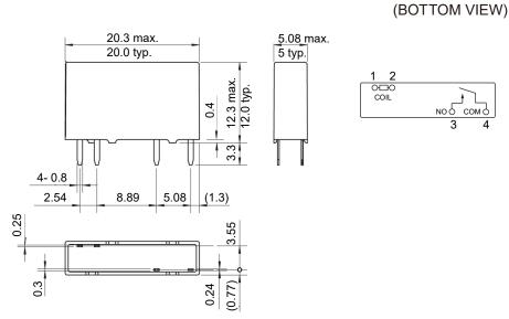
PC board mounting hole layout (BOTTOM VIEW)
