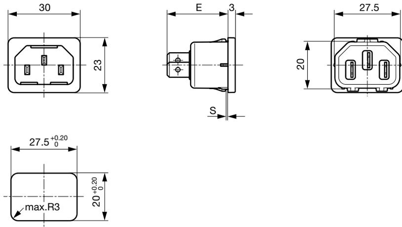
E: Lötanschlüsse 22.5 mm
